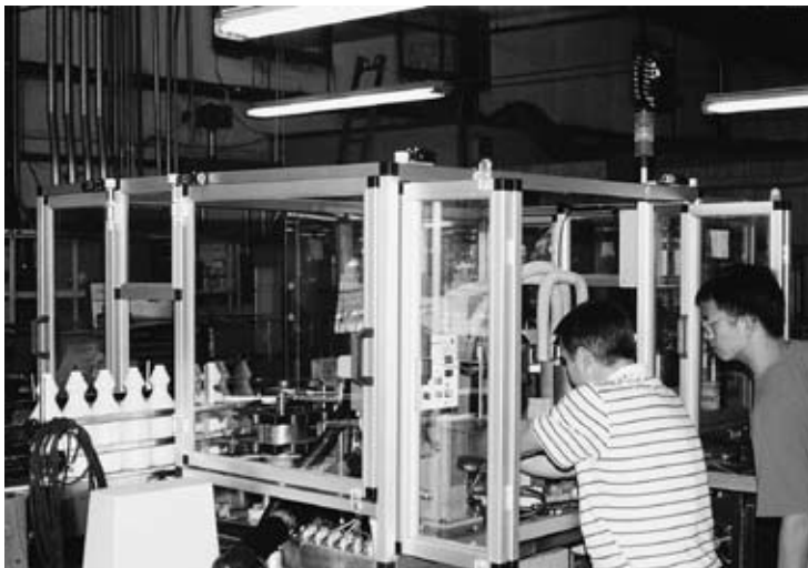
FlexTech's many extrusion profiles provide the flexibility to engineer several types of doors and panels on this labeling machine.
