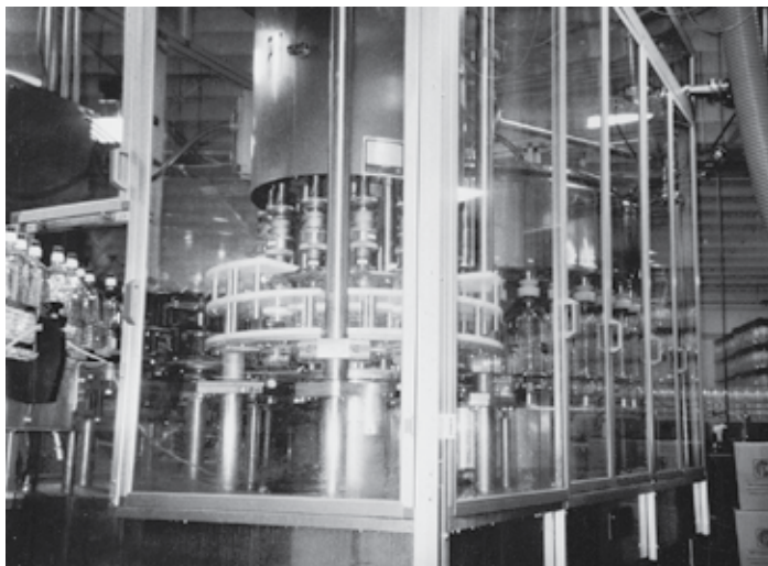
This filler uses 6 ft. high bifold doors to fully enclose the star wheel while permitting unobstructed access.
